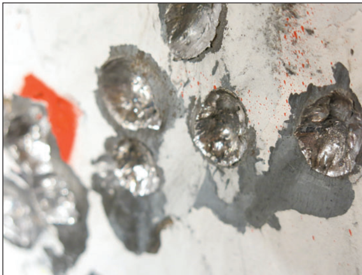
Figure 10 —Cratering of AR-500 steel plate by steel core bullets was visible at high impact angle (60-80 degrees from horizontal) but not at low angles (20-40 degrees from horizontal).
