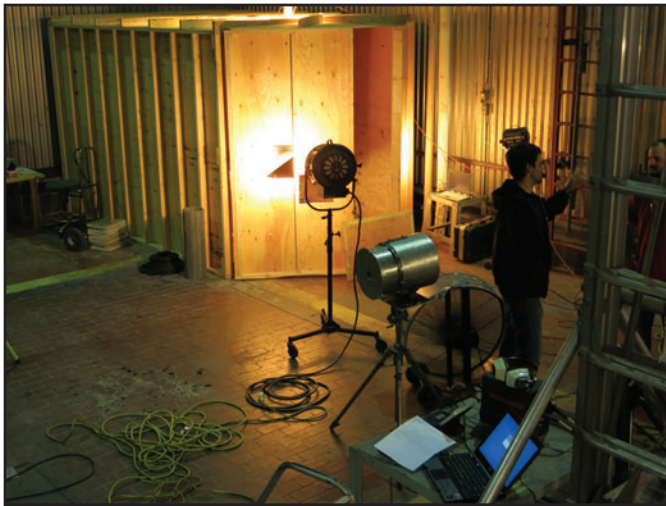
Figure 7 —Bullet trap was housed in a plywood shell to shield laboratory equipment from stray fragments. Windows were cut in the doors for lighting and cameras.
