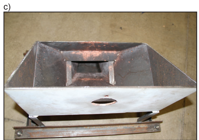
Figure 9 —Photographs of the “birdhouse” attachment to the deflector plate on the bullet trap that allowed collecting and concentrating fragments onto plates painted with temperature sensitive paints: (a) Front view showing hole through which the bullet passes, (b) side view showing baffles and funnel, (c) top view showing location of plate in the bottom of the funnel.
