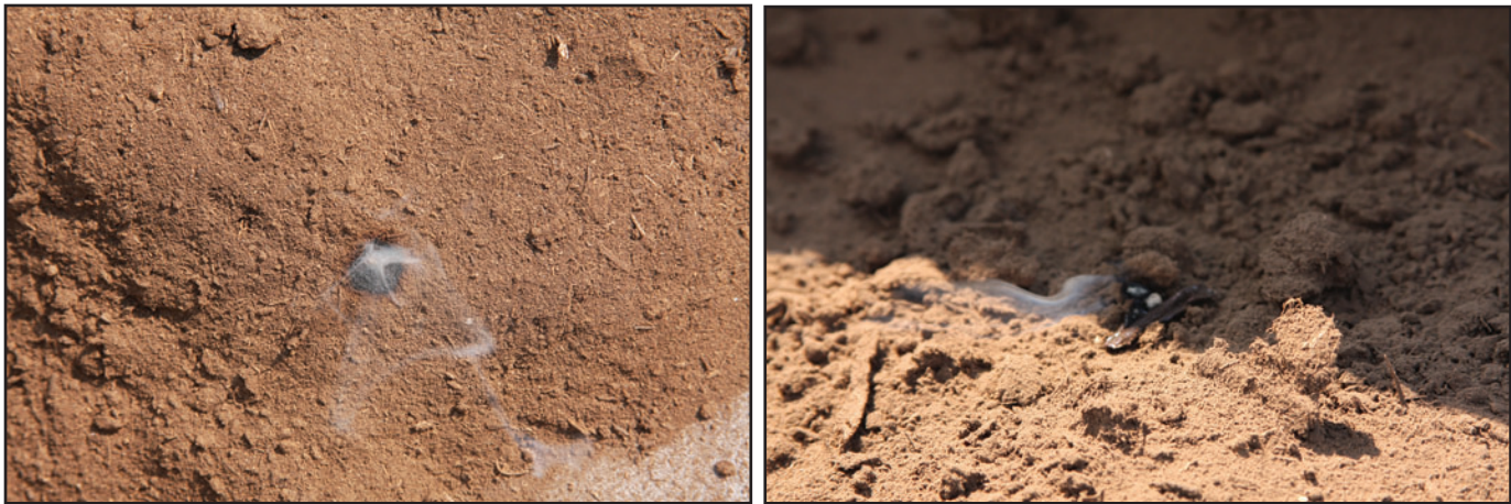
Figure 8 —Photograph showing smoldering ignition from a hot bullet fragment as first detected in the peat. Smoldering spots are approximately 1 cm in diameter (0.4 inches).
